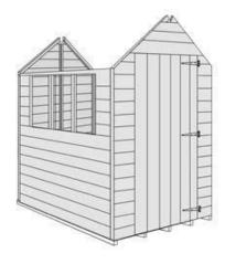
The shed front panel may now be attached to the two side panels in a similar manner to that used for the sides and back panel.
