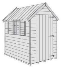
The shed roof is then finished by tacking the roof felt in place with galvanised 'clout-nails', attaching barge boards across the apex of both the front & rear panels. Finials are now added to cover barge board joins.
