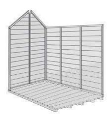
The back panel may then be placed onto the floor, together with the first side panel, prior to joining these panels together in three places – top, middle and bottom, using the 4" screw bolts and washers provided. Following this, the second shed side panel is attached to the shed back panel in a similar manner. Do not screw or nail these panels to the floor at this stage as it could restrict movement of the building when securing the roof panel.
